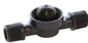
TLCV Inline Check Valve • Flow Range: 0.9 to 4.4 GPM • Opening Pressure: 10.2 psi • Closing Pressure: 5.8 psi (13.4 Feet Column of Water)
