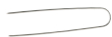
6" Soil Staple (Place approximately every 3'-5' of tubing, plus two on each tee, elbow or cross) Model TLS6
