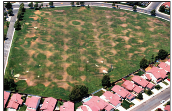
Aerial view of sports field with severe 'donuts' caused by rotary sprinklers
