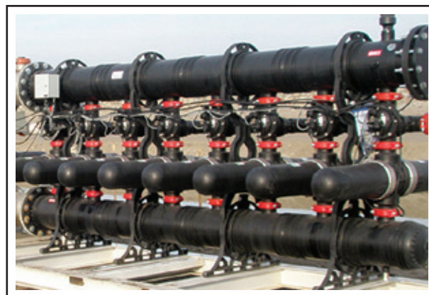
Figure 3. An example of a Netafim Apollo Disc Filtration unit (left) and Manual Disc Filter (right).
