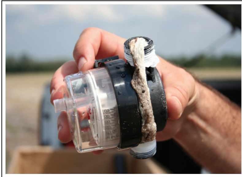
Figure 11. Filamentous sulfur slime completely clogging a small water meter.
