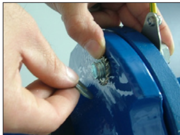
STEP 8 Add the flat washer on top of the serrated washer.
