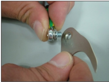
STEP 4 Attach to the Fork Terminal Lug and tighten (as shown in all three pictures).
