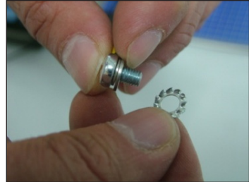
STEP 3 Insert the serrated washer on the flat washer.
